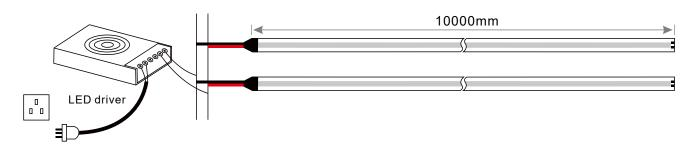
Parallel connection is highly recommended for safe electrical operation.
