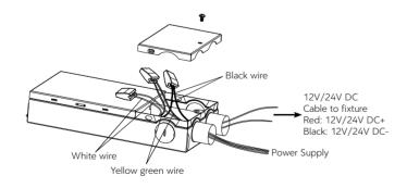
Install the strain relief bushing in the appropriate hole, then push the wires through the connector.
