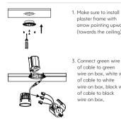
plaster frame with arrow pointing upwards (towards the ceiling)
