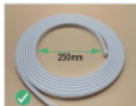
Each roll is 5 meters. When packaging (reeling), cut inward as shown, maintaining a minimum bending diameter of 250mm.
