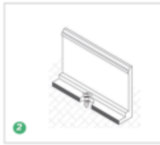
Place the clips in position and secure them with screws.
