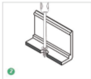
2 Place the clips in the correct position and secure them with screws.
