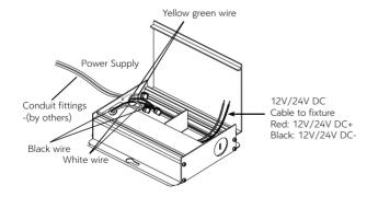
Install the strain relief bushing in the appropriate hole, then push the wires through the connector.
